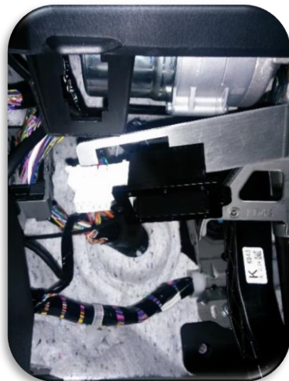
Remove OBD jack by pressing down the lug
