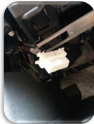
Remove the retaining clip from the plate
