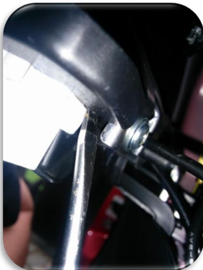
Remove OBD jack by pressing down the lug
