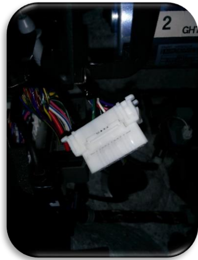
remove the plastic lug on the OBD jack
